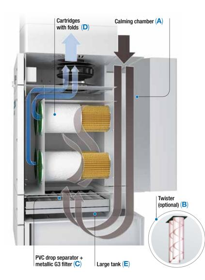
The air entry section, which connects the piping to the filter, consists in a large area which serves as a calming chamber (A). Inside this area a pre-blasting system "Twister" (B) (optional) can be provided, which further facilitates the aggregation of the finer particles by means
